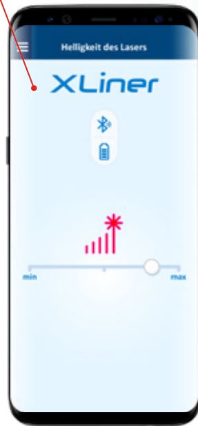
ADJUSTMENT OF THE LASER BRIGHTNESS
